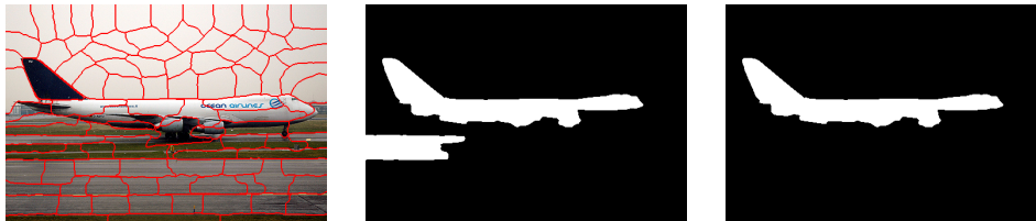
Figure 13. Image/CRF/CRF+conn. Connectedness can remove clutter: local evidence (edges on the runway) is overridden.
